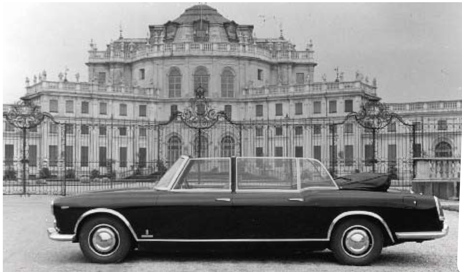
Above: elegant side profile of Flaminia 335; 3.35m wheelbase gave rise to name. GM helped with design, supplying electrics for the hoods; all could seat seven, with folding occasional seats in Connolly hide-trimmed cabin. Far right: passing Colosseum – mounted escort was appropriate because the cars were named after horses: Belfiore, Belmonte, Belsito and Belvedere
