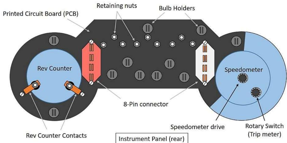
Two nuts secure the rev counter to the PCB and another nine small retaining nuts attach it to a pod containing the three gauges (fuel, water and oil). These nuts also mark the points where the instruments make electrical contact with the hidden face of the PCB. Once all of the nuts and six self-tapping screws have been removed, the PCB can be lifted off and inspected.
