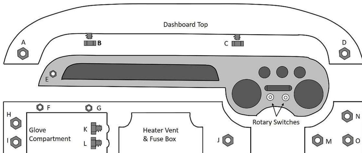
To gain access to the instruments, only the dashboard top must be removed. However visibility and access to retaining nut C is greatly improved if the lower panels are also removed or loosened.
