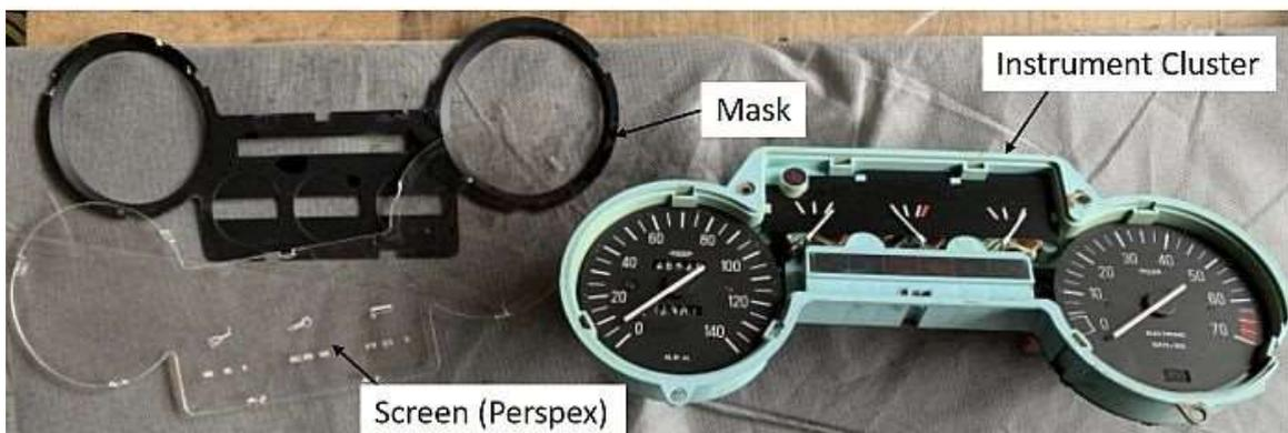
The Perspex screen is removed from the cluster by using a small screwdriver to gently lift its tabs **from the rear**, after which the mask can be lifted off. These can be cleaned, polished and retouched as necessary.
