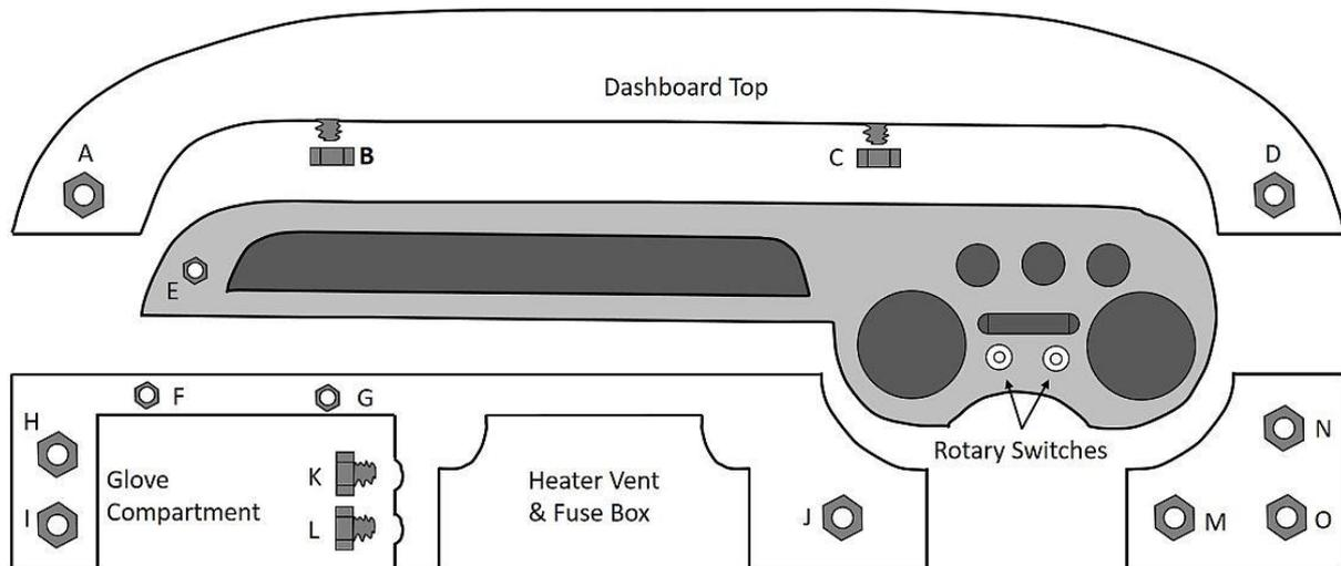
The process starts with removing the lower plastic panel of the steering column (4 long screws) and the right-hand panel of the lower dashboard, which is held by three nuts (M-O) behind the panel. Nut M attaches the panel to a small bracket near the steering column. At this point, nut D can be removed.
