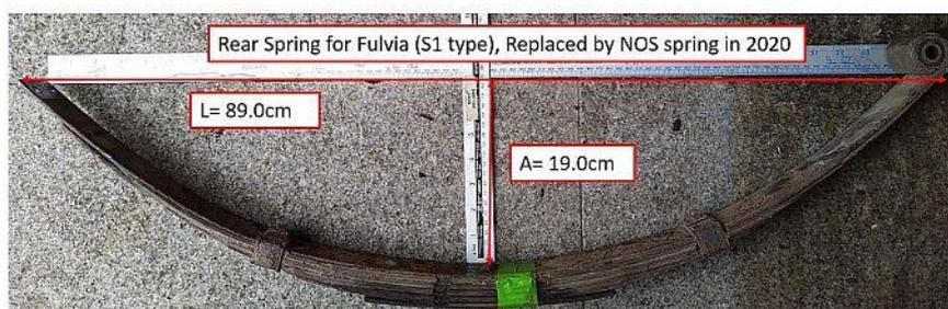
The NOS springs shown were obtained in 2020 with their factory paint and stencilling intact and so, in order to preserve this and prolong the life of the spring, some thought was given to their protection while in use. The use of spring gaiters was considered but rejected, since any failure of the seal leads to the trapping of water and enhanced, unobserved corrosion.
