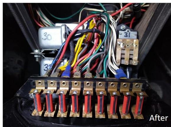
After disassembly, the fuse block, relays, contacts and spade connectors were cleaned with wire wool and fine emery paper. Wires can be cleaned with solvent (isopropanol or white spirit).
