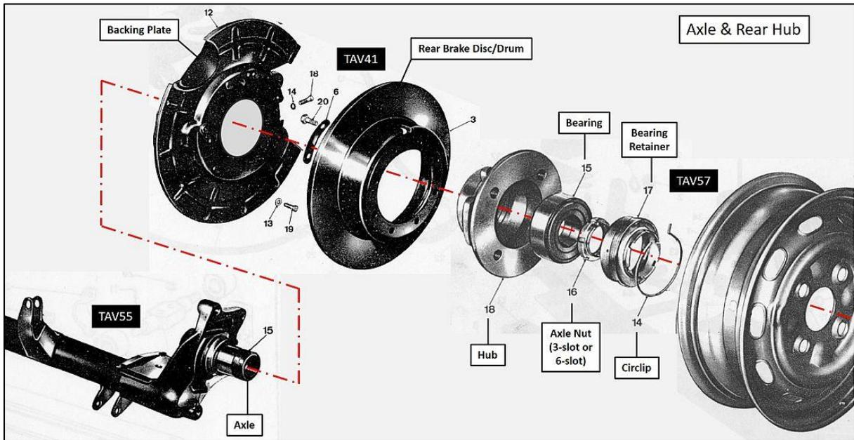
The bearing retainer and the axle nut have fine threads and are difficult to remove when dismantling the hub to change the bearing or gain access to the brake drum. Special Lancia tools are available and should be sought out, but usually need to be used in conjunction with (or welded to) a long bar. Note that 3- and 6-slot versions of the axle nuts were used by Lancia on both front and rear axles and it is important to know which are present on your car.
