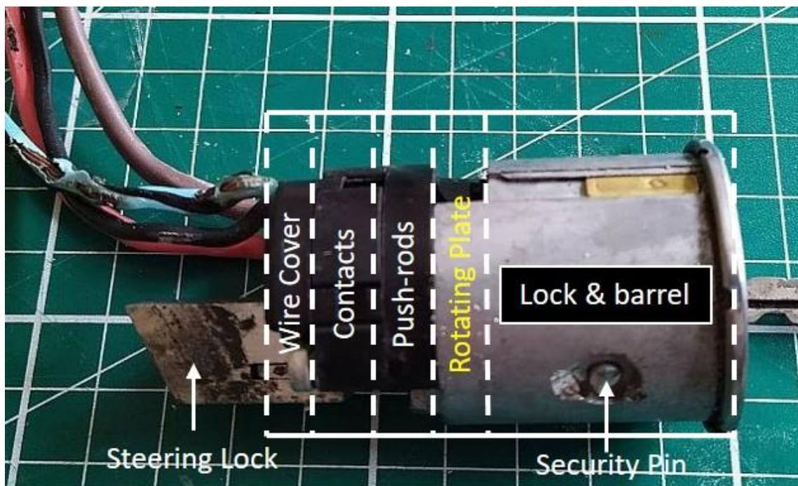
After removing the two long screws, the plates holding the contacts and push-rods can be withdrawn separately. Care must be taken not to lose the small (2mm x 8mm) push-rods which should be free to move in their plate. Note that, when assembled, the rounded ends of the push-rods face towards the rotating plate, while their flat ends rest on the contacts.
