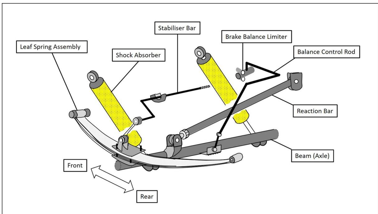
The layout of the rear suspension is shown in the diagram above. Sideways motion of the Beam (Axle) is limited by a sturdy Reaction Bar (also called a Panhard Rod) which is hinged at both ends to
