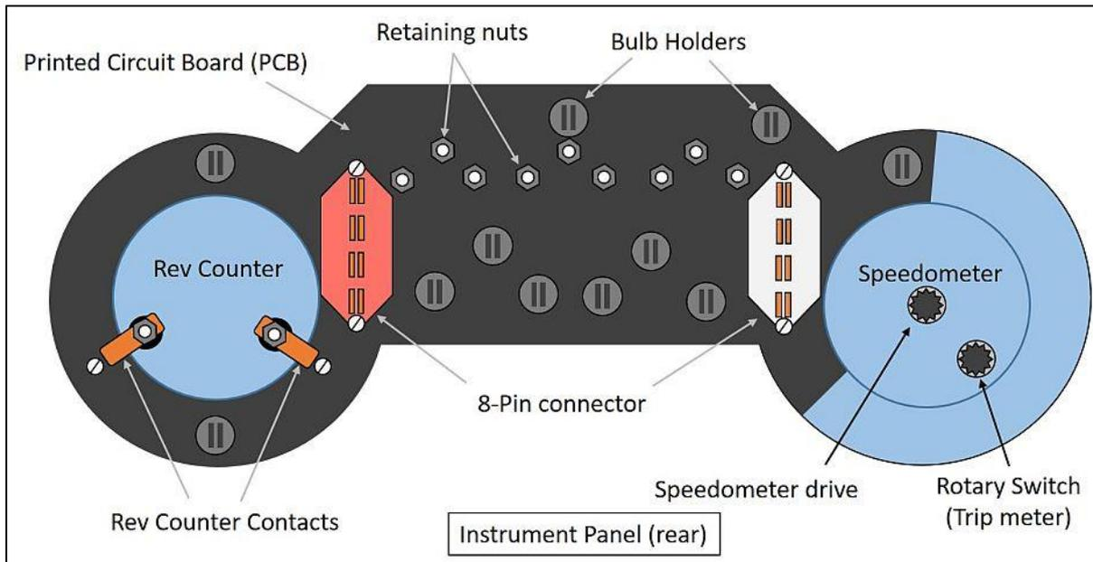
Two nuts secure the rev counter to the PCB and another nine small retaining nuts attach it to a pod containing the three gauges (fuel, water and oil). These nuts also mark the points where the instruments make electrical contact with the hidden face of the PCB. Once all of the nuts and six self-tapping screws have been removed, the PCB can be lifted off and inspected.
